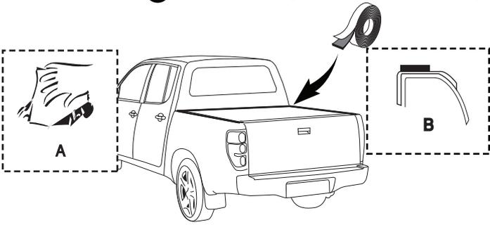
**C** Put the hardtop on top for the sponge seal and align left and right properly.
