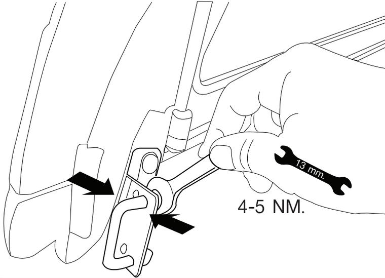
**F** Align and adjust with 2 steps rotary lock system.
